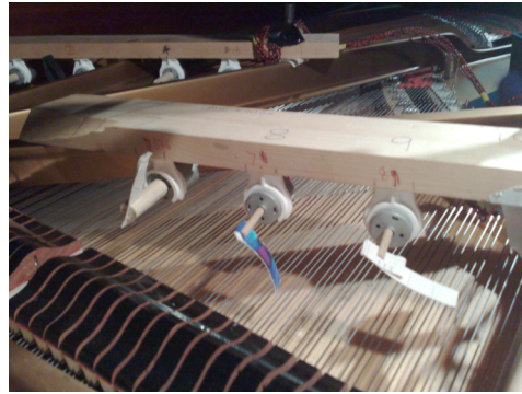
Figure 3. DC motors in the piano.
